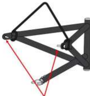
2x Upper Gantry Bolts, M6 x 35mm, 316 SS.
